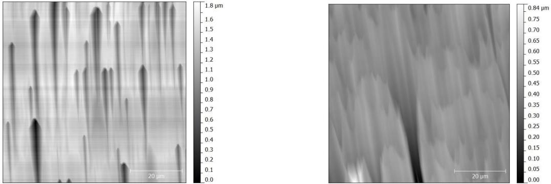
Figure 3. AFM measurements of two samples dry-etched with Ni-Au mask and different inclination angle in the RIE reactor of 0° (left) and 10° (right), c.f. Tab. 2.
