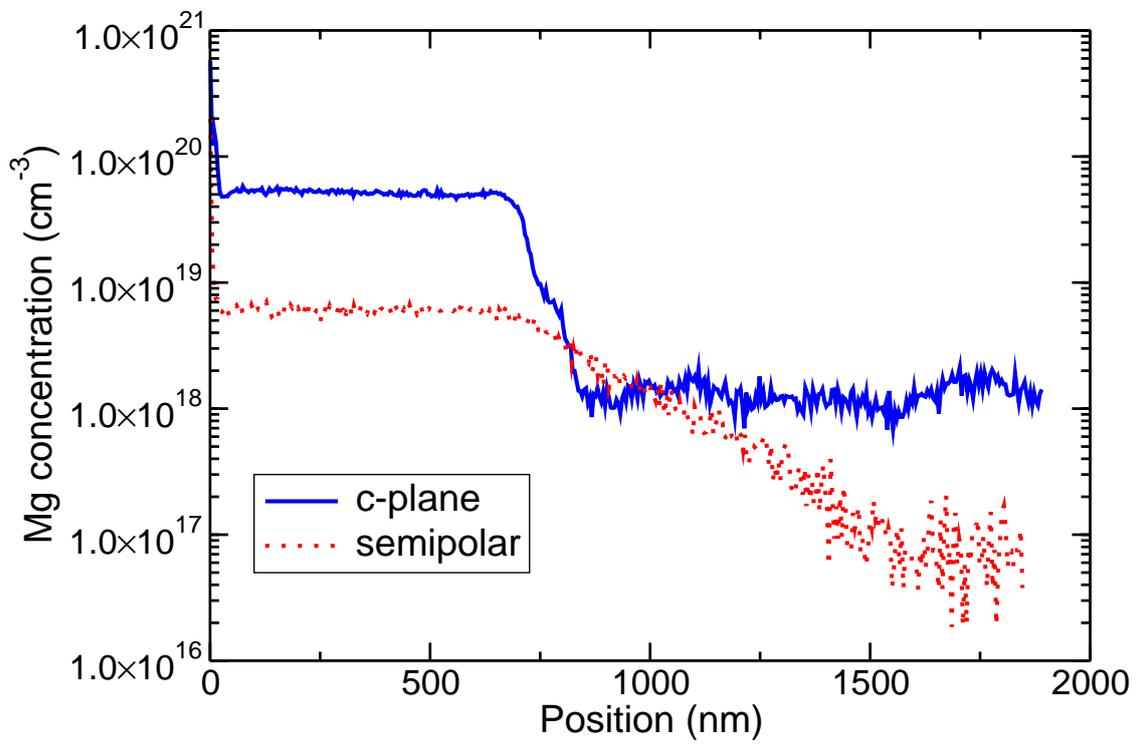
Figure 9. SIMS profiles of a c-plane and {11 $\bar{2}$ 2} semipolar GaN:Mg layer grown side by side in one run.
