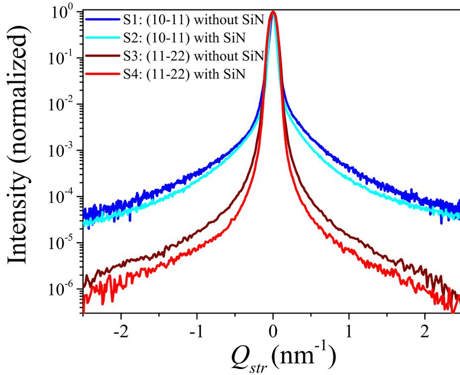
Figure 6. Intensity distribution along stacking fault streaks of semipolar GaN layers with  $\{10\bar{1}1\}$  and  $\{11\bar{2}2\}$  surface grown with and without a SiN nanomask interlayer, as indicated in Tab. 4.
