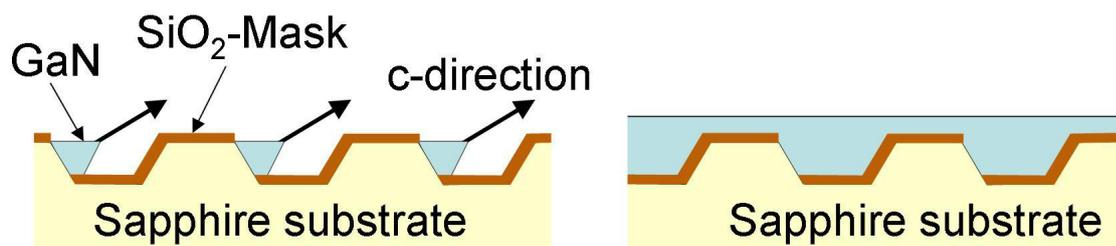
Figure 1. GaN growth nucleating at the inclined *c*-plane-like sidewalls of grooves etched into a foreign substrate (schematically). The growth first proceeds in *c*-direction (left), later the single stripes coalesce by lateral growth eventually forming a semipolar surface (right).
