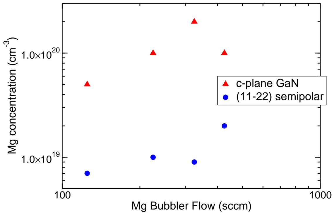
Figure 8. Mg concentration measured by SIMS versus  $\text{Cp}_2\text{Mg}$  precursor flow in c-plane and  $\{11\bar{2}2\}$  GaN:Si layers grown side by side in the same runs.
