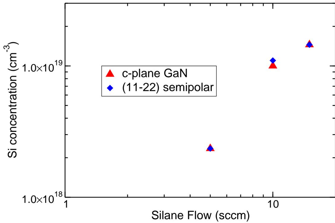
Figure 7. Si concentration measured by SIMS versus SiH<sub>4</sub> precursor flow in c-plane and {11 $\bar{2}$ 2} GaN:Si layers grown side by side in the same runs.
