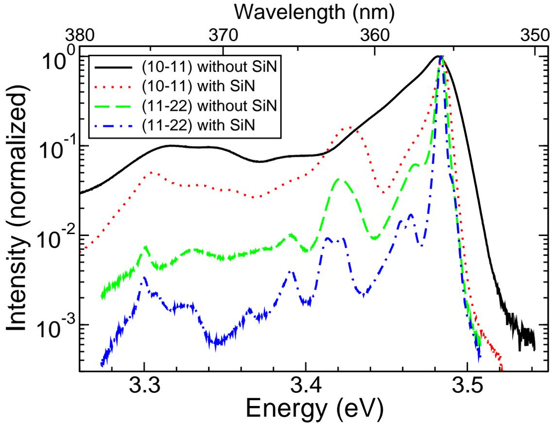
Figure 5. Low-temperature photoluminescence spectra of semipolar GaN layers with  $\{10\bar{1}1\}$  and  $\{11\bar{2}2\}$  surface grown with and without a SiN nanomask interlayer, as indicated in the figure.
