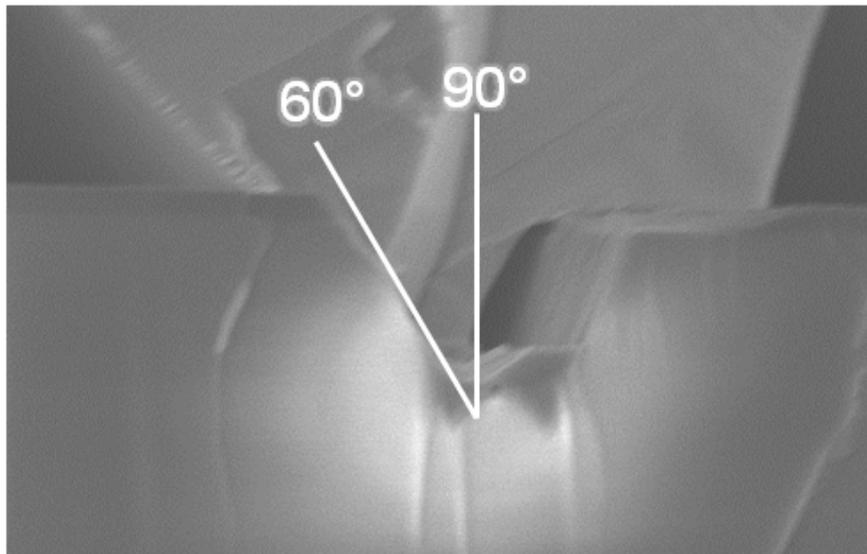
Figure 2. Trench etched after tilting the sample in the dry-etching chamber by 10°. A facet angle of 60° was obtained.
