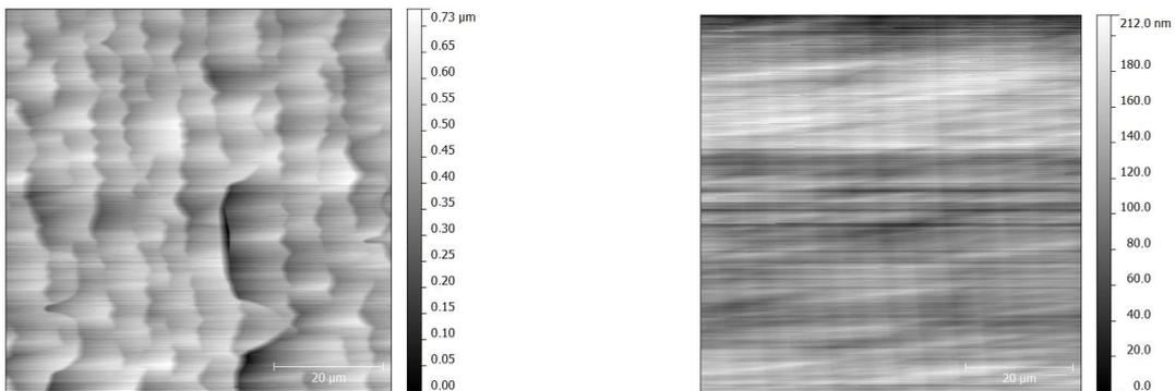
Figure 4. AFM measurements on two samples etched with photoresist mask under different RIE reactor pressure of 1.3 hPa (left) and 5.3 hPa (right), c.f. Tab. 3.
